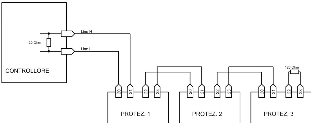
It is suggested to terminate the serial line with a resistance 120 Ω, 1/4 W.
