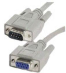
To connect PC and RGDAT-A70 you must use a "straight" serial cable, such as the one shown in the figure.
